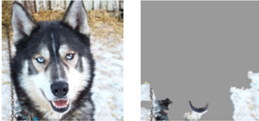
Figure 6-7: Left: Husky Classified as Wolf, Right: Explanation of the Model's Prediction in the "Husky vs Wolf" Task. The prediction is correct but was caused by the presence of snow in the background. Reproduced with permission from the author. The original can be found in Ref. [27].
