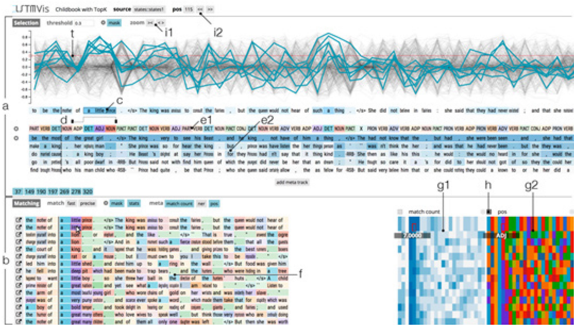
Figure 6-4: LSTMVis User Interface. The user interactively selects a range of text specifying a hypothesis about the model which is then used to match similar hidden state patterns. Reproduced with permission from the author. The original can be found in Ref. [18].
